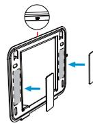
Attach the tape on the back of the Wall Mount Bracket, and attach the bracket at the desired height on the glass with the TOP logo side facing up.
