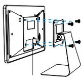
Plug an Ethernet cable into the Ethernet port of the IoT Display. Then lift the IoT Display and align its VESA holes with the VESA desktop stand.
