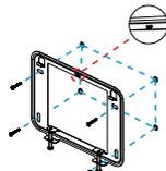
Press the bracket on the wall with the TOP logo side facing up and align its holes with the wall plugs, then fix the screws into the wall plugs.
