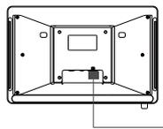
Plug an Ethernet cable into the Ethernet port of the IoT Display.
