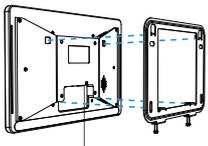
Mount the IoT Display on the Wall Mount Bracket.
