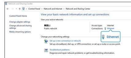
B. Go to "Properties" → "Internet Protocol Version 4 (TCP/IPv4)" and select "Use the following IP address", then assign a static IP manually within the same subnet of HL31-L08AF-915M.
