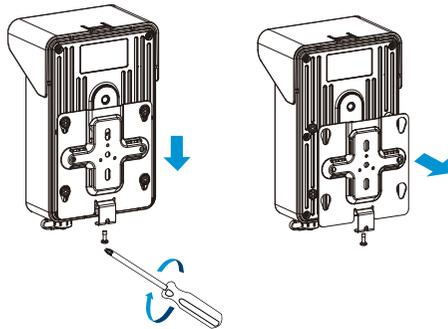
**Step 2:** Fix the backplane in the position where the device is intended to be installed. Multiple installation methods are available depending on the installation location:
