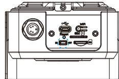
**Step 2:** Press the Wi-Fi button to enable Wi-Fi of the device.
