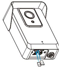
**Step 5:** Cover back the Interface Panel and fix the screws.
