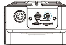
**Step 3:** Use mobile devices or laptop to connect to the device's Wi-Fi.
