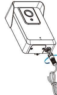
**Step 7:** Connect the device to the Installed Backplane and tighten the fixing screws. The installation is completed.
