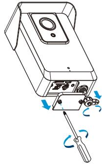
**Step 4:** Insert the SD Card and SIM Card.
