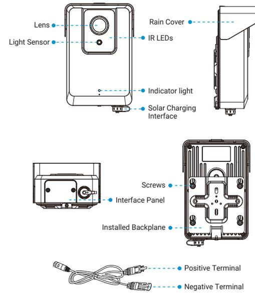
**Note:** The Positive Terminal of the Solar Panel Cable needs to be connected to the Negative Terminal of the solar panel, and the Negative Terminal needs to be connected to the Positive Terminal of the solar panel.
