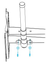
2. Connect one end of the antenna coaxial cable to the LoRaWAN® antenna, the opposite end to the device's antenna connector.
