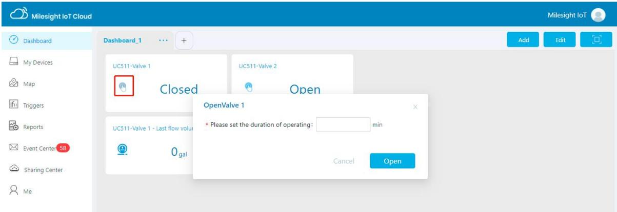
**Note:** If the working mode of UC51x is LoRaWAN® Class A, control commands will delay until the time icon disappears.
