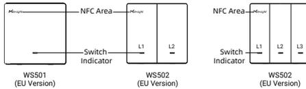
**Reset to Factory Default:** hold on any switch for more than 10s until indicator quickly blinks.
