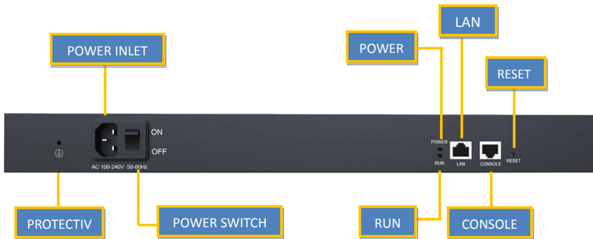
Figure 2-6 NeoGate TG1600 Rear Panel
