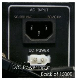
Figure 4 External D/C Power Input
