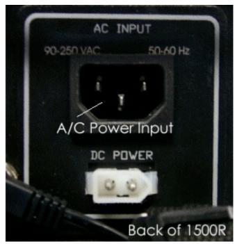
Figure 3 External A/C Power Input
