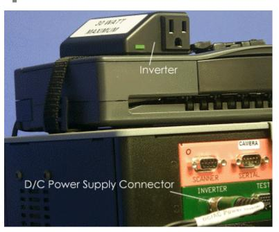
Figure 5 Power Inverter Panel
