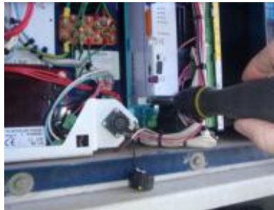
Secure 2 torx screws
