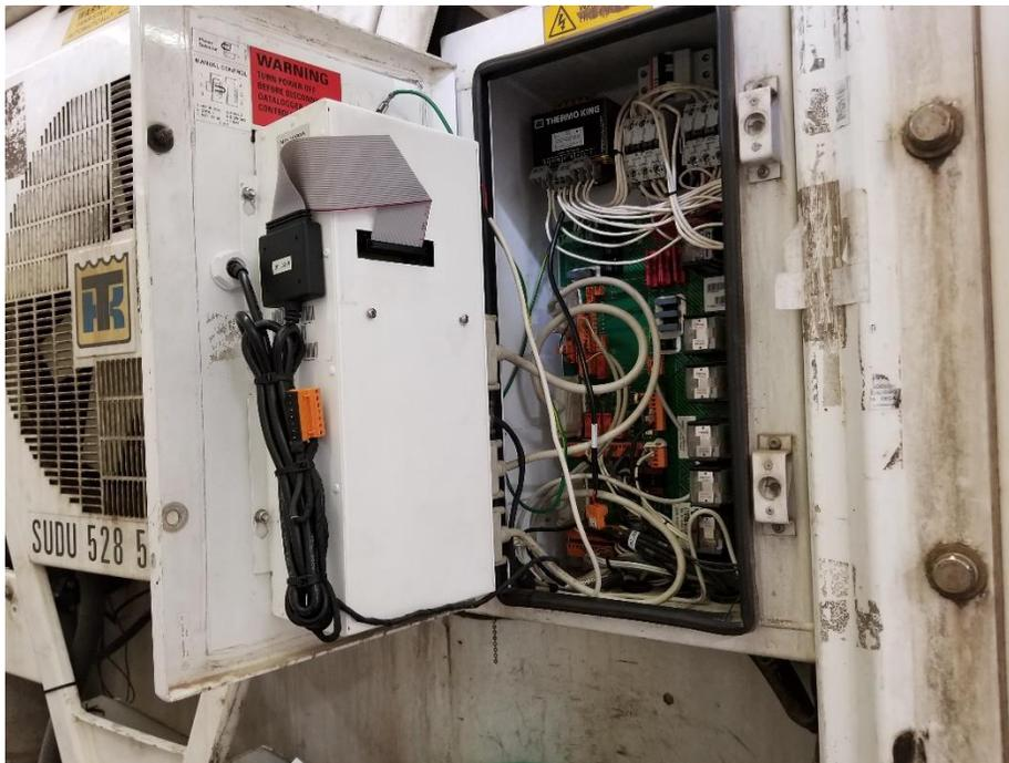
11. Close the asset door. The device should be oriented as pictured below:
