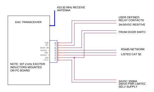
eAC System components are designed to meet the requirements for Class 2 circuits operating from a non-hazardous secondary power source limited to 240 VA. Cabling materials must be selected for the installation environment in accordance with the applicable jurisdictional codes.
