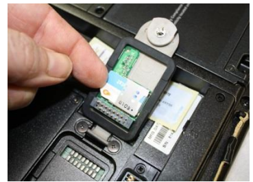
Installing a SIM card
