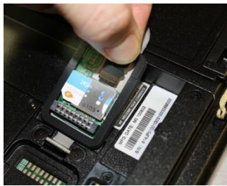
Installing a MicroSD card
