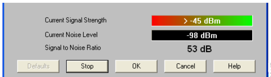
Figure 7-8 Bottom of Linktest Screen (with Test Running and Signal Strength in dBm)
