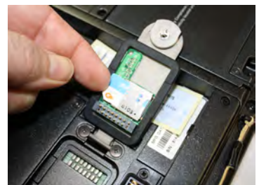
Installing a SIM card
