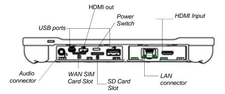
The connectors on the side of the computer are located behind the outer doors.
