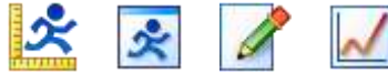
Figure 23: The workflow toolbar gives the user an optimal interface setup per functionality: Hardware and Fusion Setup, preview and record, playback and editing and analysis
