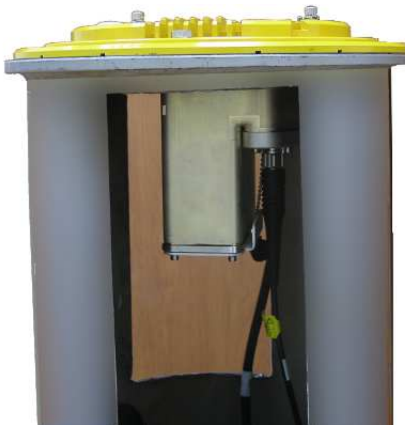
Figure 14: SDU lower unit in canister
