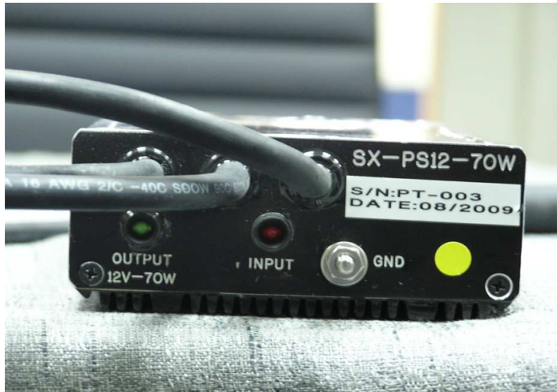
Figure 19: Power supply panel
