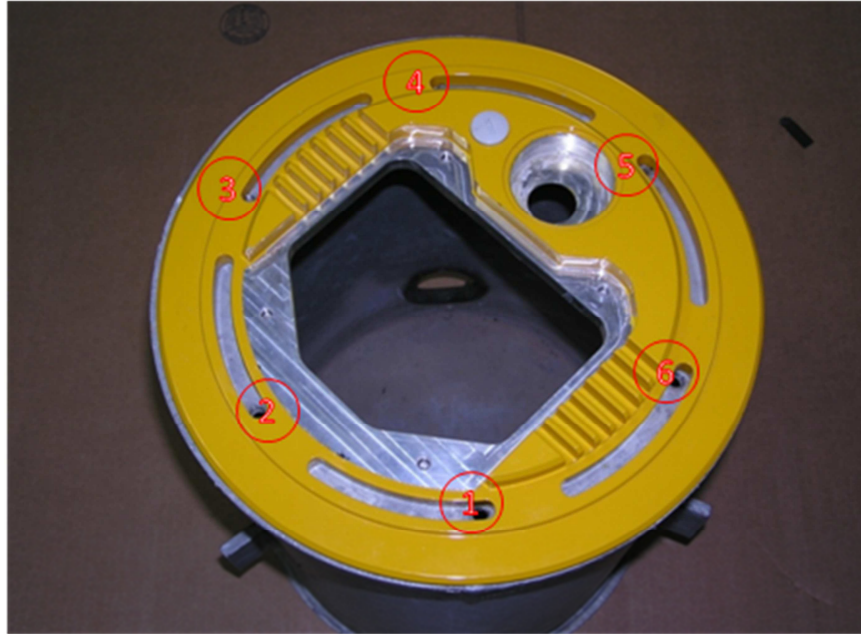
Figure 20: 12'' Canister cover screw holes
