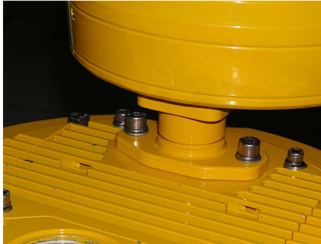
Figure 27: Sensor installed on a lower unit with screws tightened
