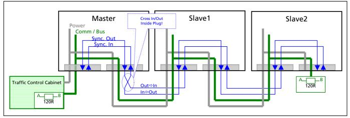
If the master unit fails, it is crucial to replace the detector as soon as possible in order for the data acquisition process to proceed. If however a slave stops working, it can be removed as long as the two connectors leading to the unit are plugged together once the unit has been removed.
