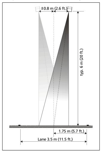
Mounting the detector left or right from the centre of the lane will likely result in less accurate traffic data.
