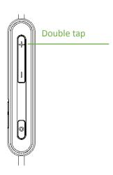
Double tap volume"+"button to switch between EN and CN language prompt under pairing mode (indicator light flashes red and blue alternatively)
