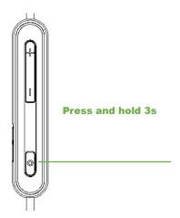
Power on -Press and hold the multi-function button(MFB)for 3s until the green light flashes;
