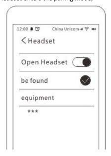
Turn on Bluetooth on your mobile, find the Model No. of the Headset, and connect. Turn off Bluetooth of the first mobile, and repeat the step above to connect with the second mobile
