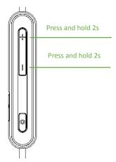
Track control - Press and hold the "Volume +" button for 2s to skip to the next song; Press and hold the "Volume-" button for 2s to play the previous song;
