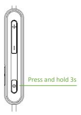
Press and hold the volume button for 3s upon charging the Headset until the green light flashes 3 times;
