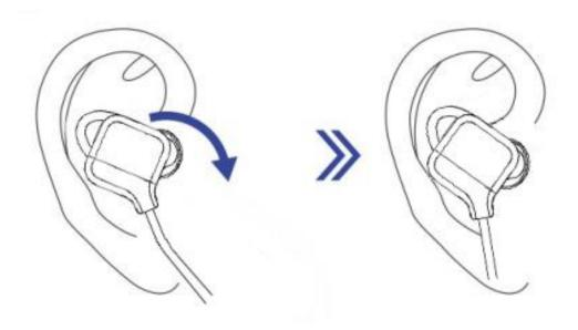
Insert the ear bud, and rotate the headset to achieve an optimal fit
