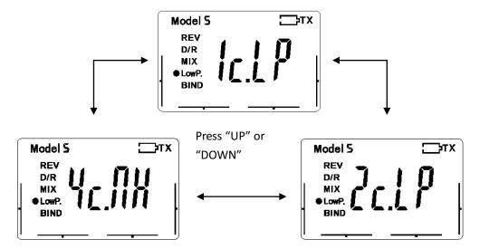
Press "UP" or "DOWN" key to change low power supply scheme, F6TB can choose 1 s lithium battery (1 c. LP), 2 s lithium batteries (2 c. LP) or 4 cell dry battery, nickel metal hydride, nickel cadmium battery (4 c. NH). Different low power supply scheme, the system will automatically adjust alarm voltage value; make sure that the users' battery won't over discharge. After confirm press "ENTER" save the setting and gets into "Bind" interface. Press "EXIT" button exit setting
