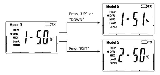
Press "EXIT" button to change the channel No., Press "UP" or "DOWN" change rudder value. Aft er confirm press "ENTER" button save setting, and enter "D/R setting" interface.
