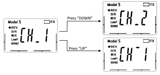
Change channel by press "DOWN", press "UP" change channel reverse setting. Please save the setting after confirm, and gets into "Dual rate setting". Press "EXIT" to exit the setting.
