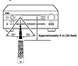
The remote control transmits a directional infrared beam. Be sure to aim the remote control directly at the remote control sensor on the main unit during operation.
