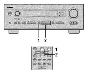
Press A/B/C/D/E (A/B/C/D/E on the remote control) to select the preset station group.
