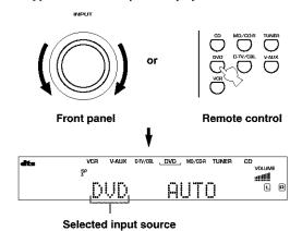
To select the audio source connected to the 6CH INPUT jacks
