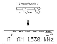
When the unit is tuned in to a station, the "TUNED" indicator lights up and the frequency of the station received is shown on the front panel display.
