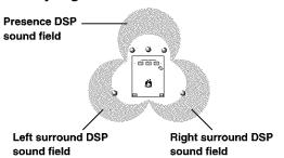
These programs use YAMAHA's tri-field DSP processing on each of the Dolby Digital or DTS signals for the front, left surround, and right surround channels. This processing enables this unit to reproduce the immense sound field and surround expression of a Dolby Digital-or DTS-equipped movie theater without sacrificing the clear separation of all channels.
