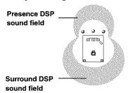
Most movie material has 4-channel (left, center, right, and surround) sound information encoded by Dolby Surround matrix processing and stored on the left and right tracks. These signals are processed by the Dolby Pro Logic decoder. The MOVIE THEATER programs are designed to recreate the spaciousness and delicate nuances of sound that tend to be lost in the encoding and decoding processes.
