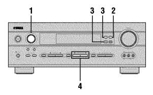
1 Rotate the INPUT selector (or press TUNER on the remote control) to select TUNER as the input source.
