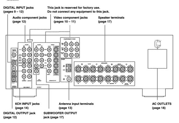
All illustrations of the rear panel in this manual are based on the HTR-5650. The jacks in the shaded area in this illustration are not present on the HTR-5640.
