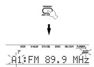
When automatic preset tuning is completed, the front panel display shows the frequency of the last preset station.
