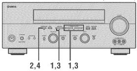
1 Select preset station "E1" using A/B/C/D/E and PRESET/TUNING
