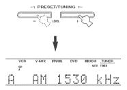
When tuned into a station, the TUNED indicator lights up and the frequency of the received station is shown in the front panel display.
