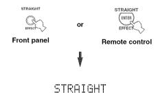
Press STRAIGHT (EFFECT) again so that "STRAIGHT" disappears from the display when you want to turn the sound effect back on.
