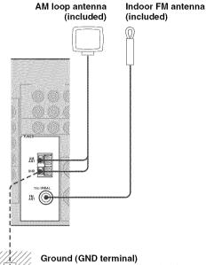
For maximum safety and minimum interference, connect the antenna GND terminal to a good earth ground. A good earth ground is a metal stake driven into moist earth.
