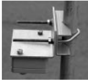
Close up of the bracket and mounting hardware attached to the amplifier.
