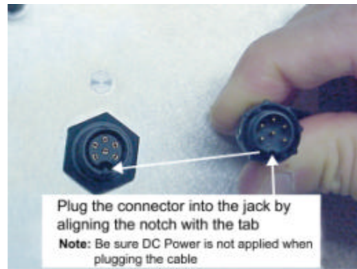
Figure 6 – Plugging the Round Connector
