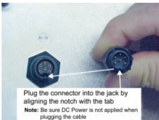
Figure 6 – Plugging the Round Connector
