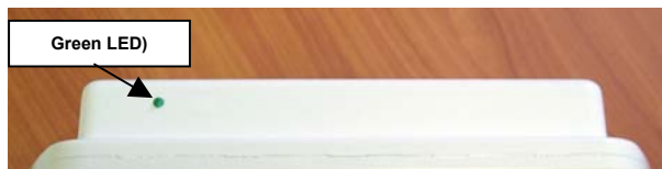
Figure 10 – Marquee Bridge LEDs
