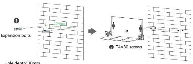
Hole depth: 30mm Hole diameter: 6mm
