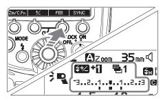
improve the success rate of photo taking. The FEB function can be set pressing function button [FEB], the FEB value can be adjusted by rotating [Dial], settings can be saved by pressing [SET] button.
