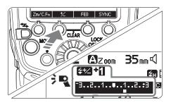
function button [+/-], the FEC value can be adjusted by rotating [Dial], settings can be saved by pressing [SET] button.
