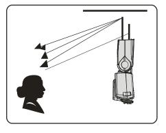
(catching light). This function can reach optimal effect when the flash head is upward 90 degrees.
