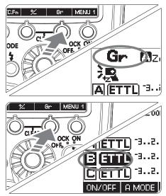
button and rotate the [Select Dial] to adjust the exposure compensation and flash output.After the parameter set press the [\_\_\_\_] button to return to the shooting ready state.
