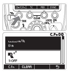
[]button back to the shooting interface. After entering the custom function menu, short press the function button [CLEAR], then short press the function button 1 [OK] will restore the custom function to factory default.
