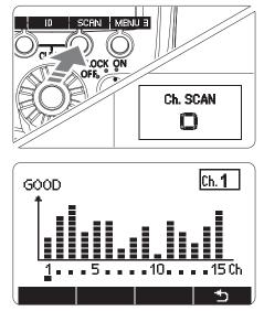
higher the peak of which channel on the chart, the stronger the radio the radio signals.
