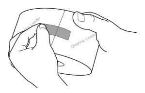
Insert the packaging paper with the metal part of the ring facing to the back of the paper core shaft.
