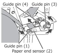
Pass the paper under the guide pin (1). Pass the paper through the paper end sensor (2). Pass the paper under the guide pin (3). Pass the paper to the left side of the guide pin (4).
