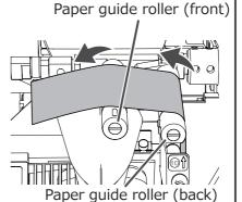
Pass the paper over the paper guide roller (back). Pass the paper over the paper guide roller (front).
