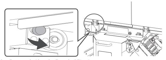
Hold the handles on each side and pull out the DTA unit.
