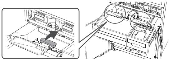
While pushing the lever back, lift the UC hopper up to release it from the pins. Then lift the DTA partition tray cover up to remove it.
