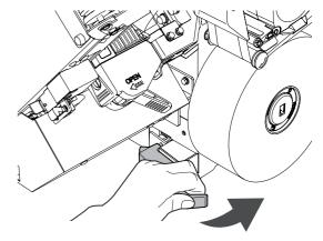
Hold the handle on the packaging unit and return the packaging unit to its original position. Push it all the way in until it clicks.
