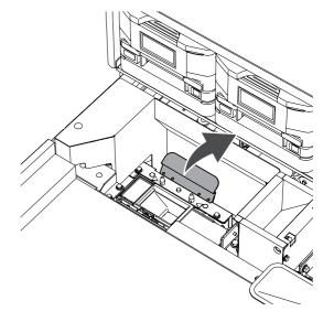
While pushing the lever back, insert the UC hopper into the pins to attach it.
