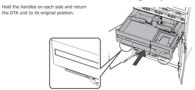
Turn the white screw which fixes the DTA unit to the right to tighten it.
