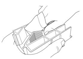
Reassemble the powder collecting unit. Assemble it by engaging tabs.
