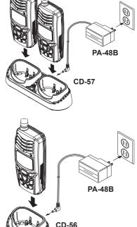
6. Remove the transceiver from the **CD-57** or **CD-57**, then unplug the **PA-48B** from the AC line outlet.
