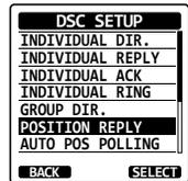
2. Press the **[SELECT]** soft key, then press the **CH▼/CH▲** key to select “AUTO” or “MANUAL”. In “AUTO” mode, after a DSC POS Request is received, the radio will automatically transmit your vessels position. In “MANUAL” mode, the display of the radio will show who is requesting the position.
