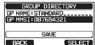
9. Press the [▲]/[▼]/[◀]/[▶] keys to select the second number of the MMSI (the first of the nine digits is permanently set to “0”) which you want to contact, then press the [SELECT] soft key to step to the next number.
