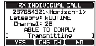
6. Monitor the specified channel until the message is completed. Press the microphone **PTT** switch and talk into the microphone to communicate with the vessel that initiated the individual call.
