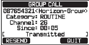
8. Listen to the channel to make sure it is not busy, then press the microphone **PTT** switch to communicate with all of the vessels in the group.
