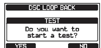
The display will show “Passed!” if the DSC feature properly operates. Press the [**OK**] soft key to return to the “DSC CALL” menu.
