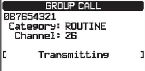
9. Listen to the channel to make sure it is not busy, then press the microphone **PTT** switch to communicate with all of the vessels in the group.
