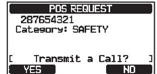
7. When the transceiver receives the position from the polled vessel it is shown on the radio display.
