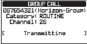
7. After the group call is transmitted, all the radios in the group will switch to the designated channel.
