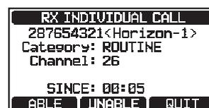
5. Press the **[YES]** soft key to send an acknowledgement. Press the **[CHG CH]** soft key to change to the requested operating channel for communication.
