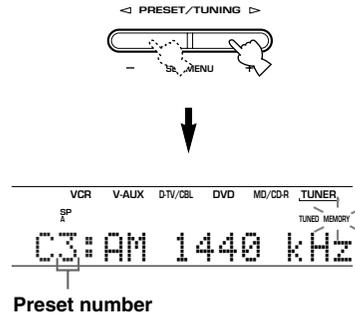
**5 Press MEMORY (MAN'L/AUTO FM) on the front panel while the "MEMORY" indicator is flashing.**
