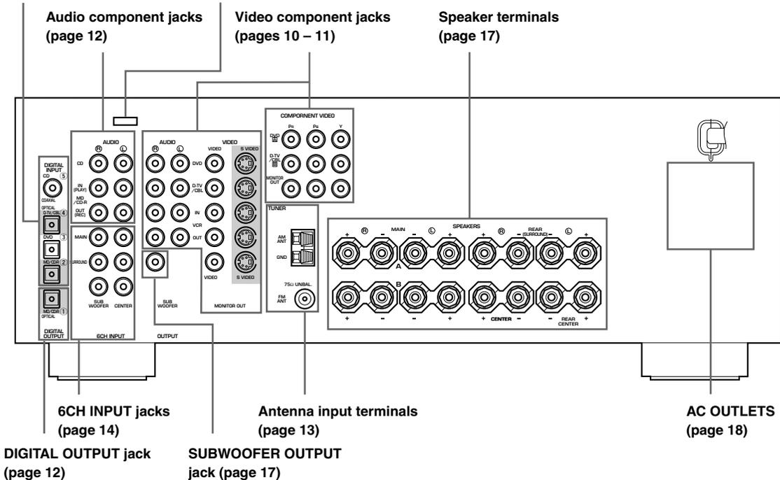
All illustrations of the rear panel in this manual are based on the HTR-5650. The jacks in the shaded area in this illustration are not present on the HTR-5640.
