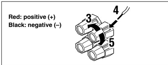
**1** Remove approximately 10 mm (3/8”) of insulation from each of the speaker cables.
