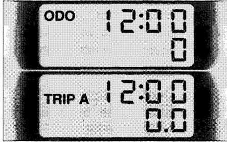
To reset the trip meter to “0”, push the mode button (left) until it displays “TRIP A” or “TRIP B”, then push the set button (right) and hold it down for at least one second.
