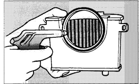
6. Tap the air filter lightly to remove most of the dust and dirt and blow out the remaining dirt with compressed air as shown. If the air filter is damaged, replace it.
