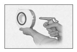
Lightly tap the air filter element to remove most of the dust and dirt, and then blow the remaining dirt out with compressed air as shown.
