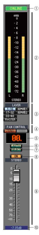
The Master window enables you to switch between layers and control Stereo Out signals. To open this window, choose [Master] from the [Windows] menu.
