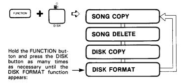
Note: If the "PROTECT!!" display appears, this usually means that the loaded disk's write protect tab is ON. Remove the disk (by pushing the button on the disk drive) and slide the write protect tab to the OFF position, then start again from the beginning of the format operation. (Pre-recorded "Disk Orchestra Collection" disks and disks recorded on a Yamaha Disklavier are specially protected and cannot be formatted).
