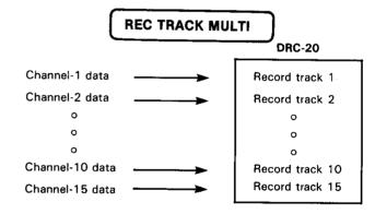
Note: The DRC-20 records data received on all 16 MIDI channels (1 through 16), and plays the data back on the same channels in this mode only.
