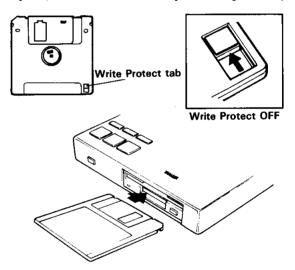
Every time you insert a brand new unformatted disk, the "Unformat DISK!!" message will appear on the DRC-20 display. This informs you that the DRC-20 cannot identify the disk you have inserted and must be formatted before it can be used with the DRC-20.
