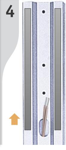
Thread **Speaker Wires** Cut speaker wire 4 to appropriate lengths for all speaker connections and set aside. Place each long stand upright on its base. Thread main speaker wire through oval opening on stand and pull through opening on underside of base. Pull wire all the way through leaving extra length near oval opening as shown. Apply non-skid
