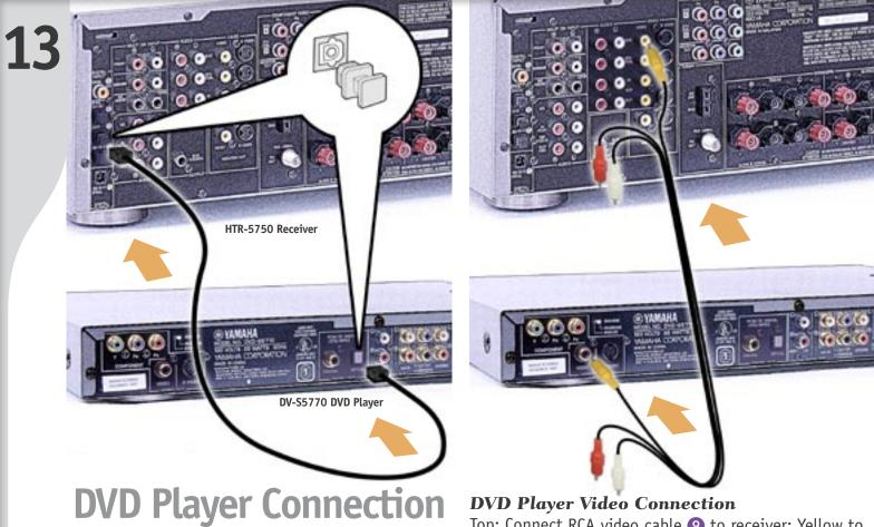
**DVD Player Optical Connection** Remove dust cap on optical input as shown on insets. Connect optical cable 10 to receiver. Connect
