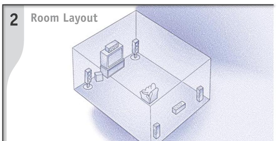
**Speaker Placement** After assembly of the speakers place them so they appear in the approximate positions as shown in the diagram above.
