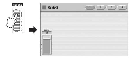
Press the [2] button at the top right of the display, then set the Type to [STAGE 1].
