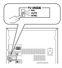
This system is designed for use with the NTSC and PAL television formats. Set this switch to the position of the format your TV monitor employs.
