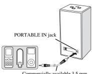
Commercially available 3.5 mm stereo mini plug cable
