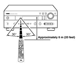
The remote control transmits a directional infrared beam. Be sure to aim the remote control directly at the remote control sensor on the main unit during operation.
