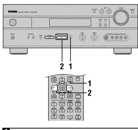
Press A/B/C/D/E (A/B/C/D/E on the remote control) to select the preset station group. The preset group letter appears on the front panel display and changes each time you press A/B/C/D/E.
