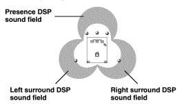
These programs use YAMAHA's tri-field DSP processing on each of the Dolby Digital or DTS signals for the front, left surround, and right surround channels. This processing enables this unit to reproduce the immense sound field and surround expression of a Dolby Digitalor DTS-equipped movie theater without sacrificing the clear separation of all channels.
