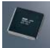
YGV-619 video processor LSI (Yamaha original)
