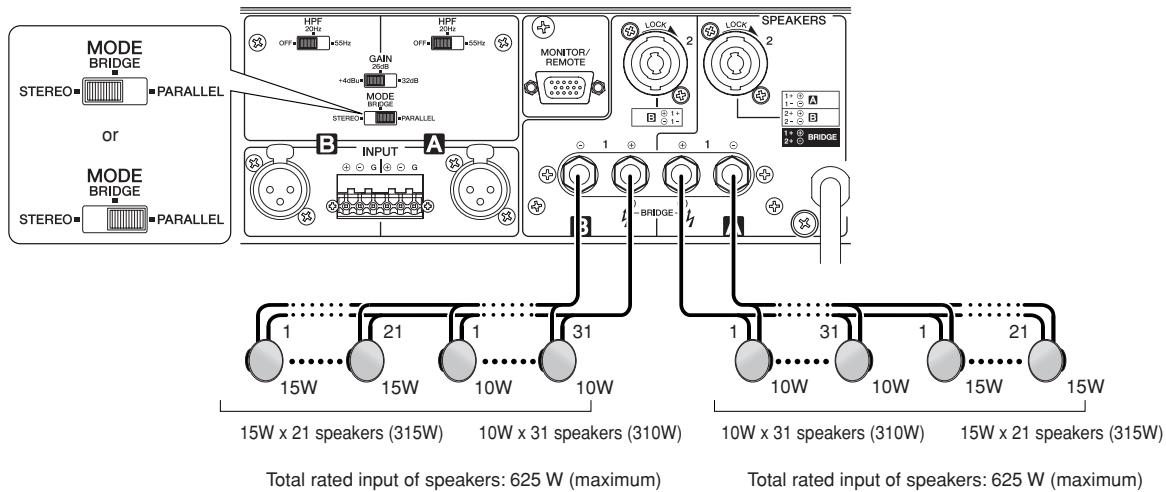
The XP3500 enables you to connect in **bridge fashion** multiple high-impedance speakers that support **100V** line output. You can connect speakers with a total rated input of up to **625 W**.
