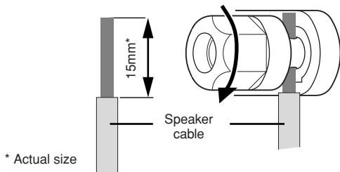
Be sure that the bare wire ends do not jut out from the terminals and touch the chassis.
