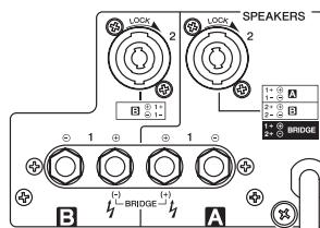
This  $\mathbb{L}$  mark indicates a dangerous electrically live terminal. When connecting an external wire to this terminal, it is necessary either to have "a person who have received appropriate guidance on handling" make the connection or to use leads or a cord that have been manufactured in such a way that the connection can be made simply and without problem.
