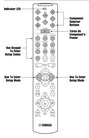
The YHT-23 Home Theater package includes a universal pre-programmed remote control with factory codes to control your HTR-5240 receiver and most Yamaha audio components. To program other brands of components (i.e., TV, VCR, etc.) or if your Yamaha unit does not respond, you will need to program the remote control with the manufacturer's codes (listed on the back pages of the *HTR-5240 Owner's Manual*).
