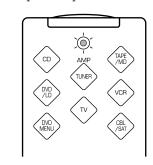
5. To verify the code works, aim the remote control at the television set, press TV, and then press POWER. The television set should turn off. If it doesn't respond, use another code for the same manufacturer and repeat steps 3 through 5.
