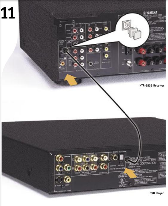
**DVD Player Optical Connection (optional)** Remove dust cap on optical input as shown on inset. Connect optical cable (not included) to receiver. Connect optical cable to DVD player from receiver.
