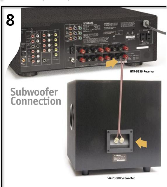
**Connect Subwoofer** Positive (+) side of the wire with white stripe attaches to (+) terminal. Negative (-) side attaches to (-) terminal.
